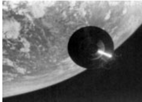
Figure 1: Speltra separation on Ariane 5 flight A-502; an image taken with a CMOS APS camera (Ref. 9).
